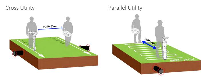
Active: With 2 users, hold the Transmitter on its side and the Locator as shown, walk the path together.
