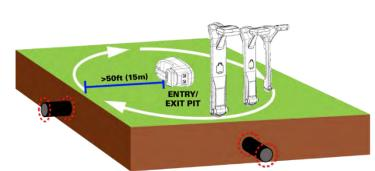
11. Move the Transmitter over each utility in turn and make Locates on other Utilities for best results.
