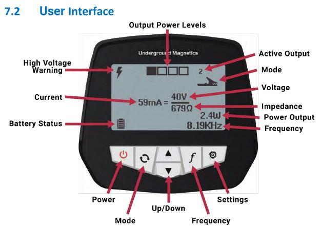
There are two main contexts for the Transmitter: **Main Screen** and **Menu Screen**. The keys can have distinct functions depending on context. The keypad is used to control the Transmitter.
