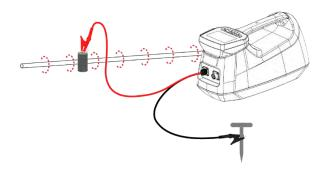
Step 2: Transmitter Direct Connection
