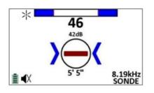
3. Move in the direction of the Sonde past the Overhead Screen to find the second Null Point.
