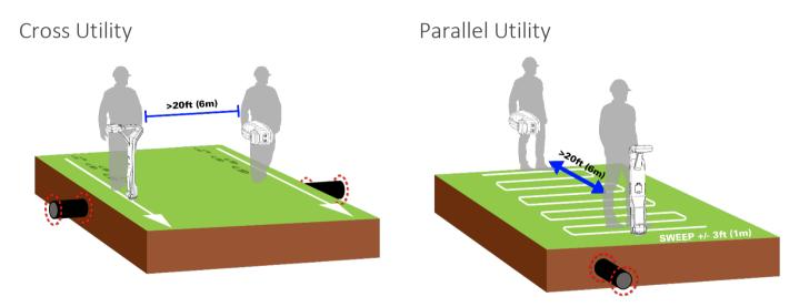
**Active:** With 2 users, hold the Transmitter on its side and the Locator as shown, walk the path together.
