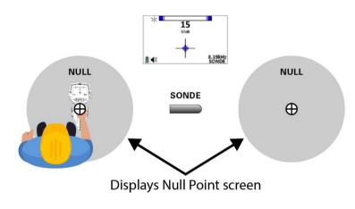
There are two different Sonde locating screens corresponding to the Null Point and Overhead areas. The Receiver automatically switches between these screens during Sonde locating. The Null Point screen will be displayed when close to a null point. The Overhead screen will be displayed when not close to a null point. The graphic below shows the areas where the Null Point screen is used.
